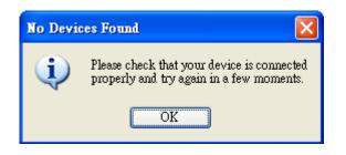
• When programming an EEPROM, a device must be selected. If no device is selected, the error message below is shown.
