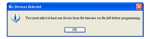
• When erasing an EEPROM, a device must be selected. If no device is selected, the error message below is shown.
