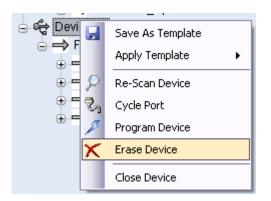
Alternatively, to erase the EEPROM of multiple devices, the user can press the program button within the toolbar or "**Devices**" menu.
