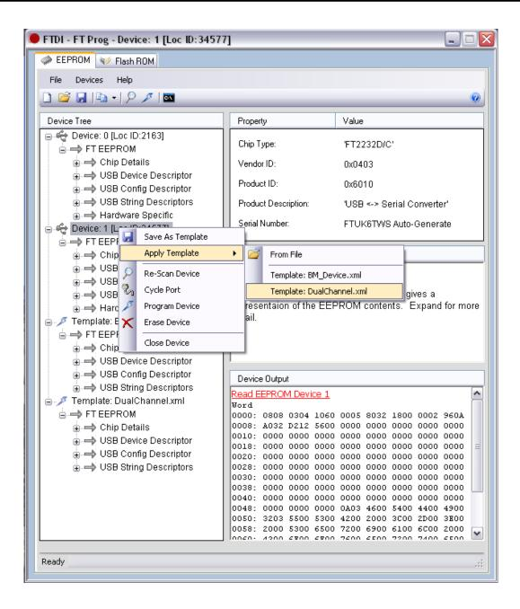
To apply a template that is not currently open within the application: right-click on the required device and select "Apply Template", "From File". This will open a file browser allowing the user to browse to the required file.
