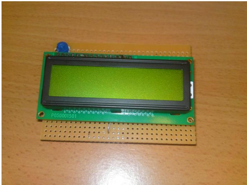
**Figure 1.2 – Topway LMB162ABC LCD Module**
