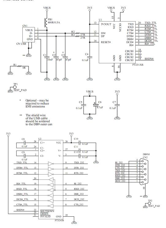
Figure 2.1 FT231XS/FT3243S Schematic
