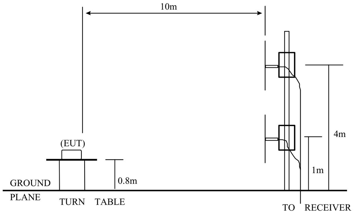
EUT = Equipment Under Test
