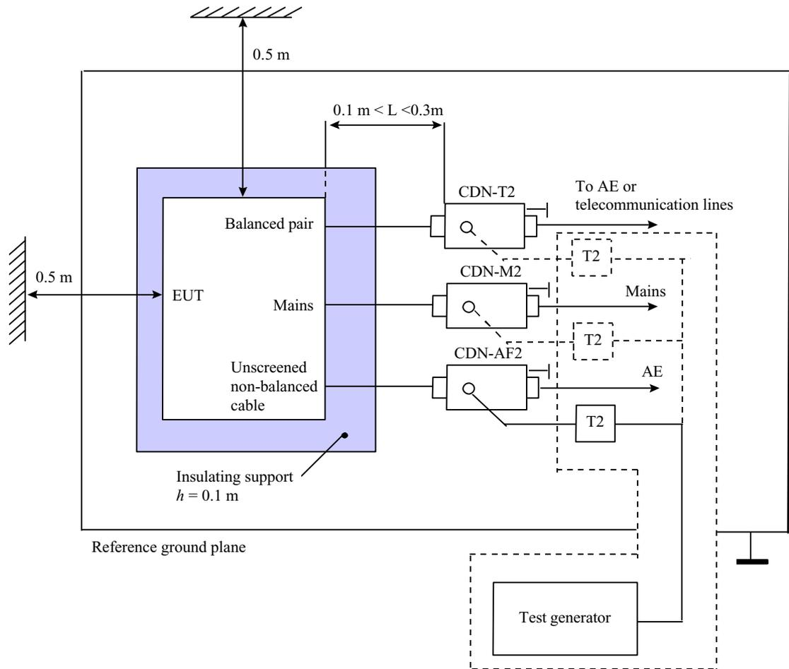
NOTE - The EUT clearance from any metallic obstacles shall be at least 0.5 m .
