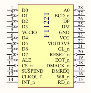
Figure 3-1 TSSOP-28 package schematic symbol
