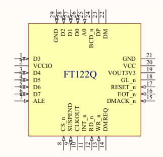
Figure 3-2 QFN-28 package schematic symbol
