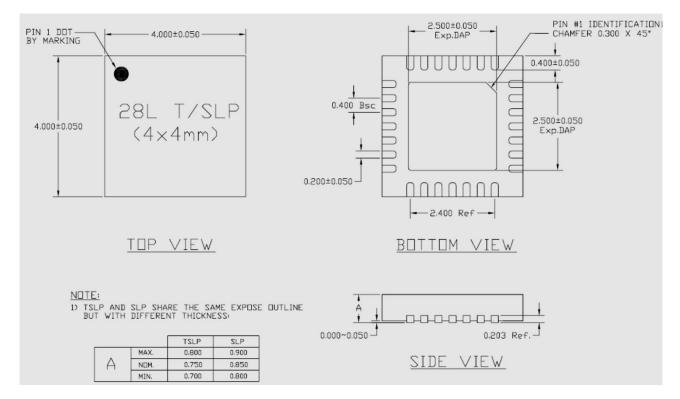
Figure 9-3 QFN-28 Package Dimensions
