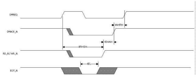
Figure 8-3 Single cycle DMA timing
