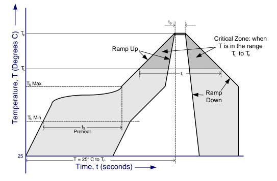
Figure 9-5 FT122 Solder Reflow Profile
