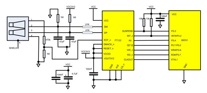
Figure 7-2 FT122 self-powered application
