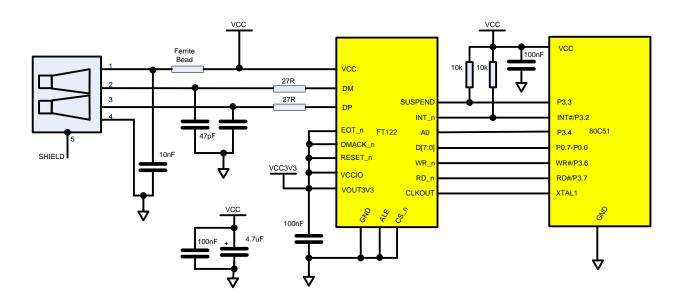
Figure 7-1 FT122 bus-powered application
