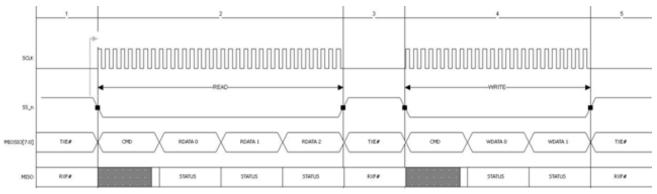
Figure 5.1: FT1248 Basic Waveform Protocol
