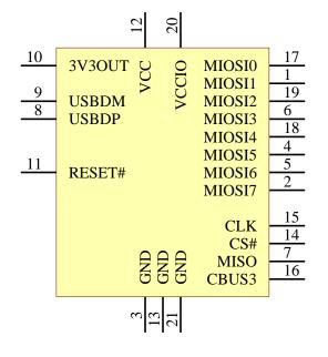
Figure 3.1 QFN Schematic Symbol
