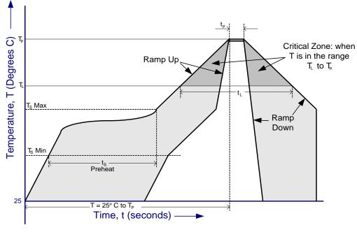
Figure 10.5 FT221X Solder Reflow Profile
