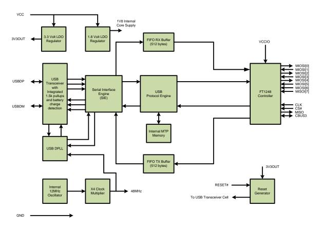
Figure 2.1 FT221X Block Diagram
