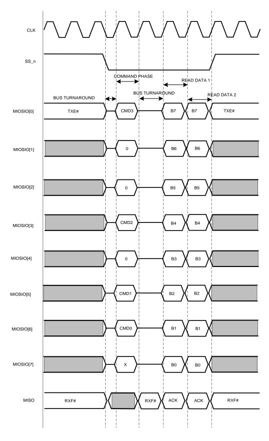
Figure 8.3 FT1248 8- bit read timing diagram
