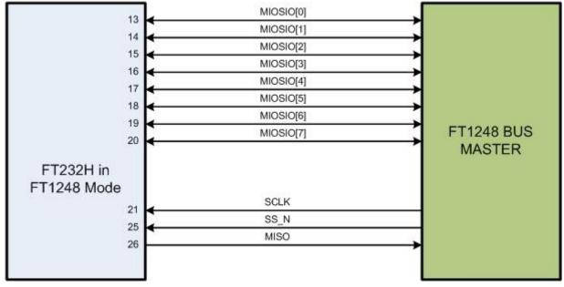
Figure 8.1 Application Example showing USB to FT1248 host
