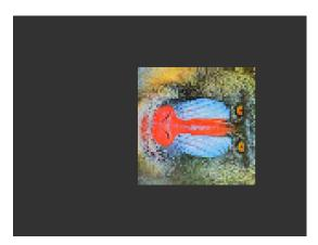
cmd(BEGIN(BITMAPS)); cmd\_loadidentity(); cmd\_translate(65536 \* 32, 65536 \* 32); cmd\_rotate(90 \* 65536 / 360); cmd\_translate(65536 \* -32, 65536 \* -32); cmd\_setmatrix(); cmd(VERTEX2II(68, 28, 0, 0));
