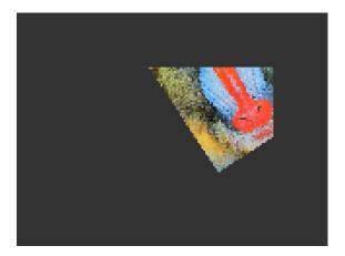
cmd(BEGIN(BITMAPS)); cmd\_loadidentity(); cmd\_rotate(-33 \* 65536 / 360); cmd\_setmatrix(); cmd(VERTEX2II(68, 28, 0, 0));
