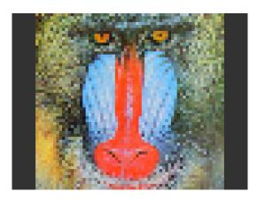
dl( BITMAP\_SOURCE(0) ); dl( BITMAP\_LAYOUT(RGB565, 128, 64) ); dl( BITMAP\_TRANSFORM\_A(128) ); dl( BITMAP\_TRANSFORM\_E(128) ); dl( BITMAP\_SIZE(NEAREST, BORDER, BORDER, 128, 128) ); dl( BEGIN(BITMAPS) ); dl( VERTEX2II(16, 0, 0, 0) );
