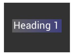
cmd(SCISSOR\_XY(20, 40)); cmd(SCISSOR\_SIZE(120, 32)); cmd\_gradient(20, 0, 0x606060, 140, 0, 0x404080); cmd\_text(23, 40, 29, 0, "Heading 1");
