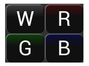
cmd\_fgcolor(0x101010); cmd\_button( 2, 2, 76, 56, 31, 0, "W"); cmd\_gradcolor(0xff0000); cmd\_button( 82, 2, 76, 56, 31, 0, "R"); cmd\_gradcolor(0x00ff00); cmd\_button( 2, 62, 76, 56, 31, 0, "G"); cmd\_gradcolor(0x0000ff); cmd\_button( 82, 62, 76, 56, 31, 0, "B");
