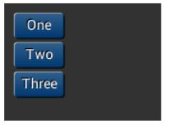
cmd\_button(10, 10, 50, 25, 26, 0, "One"); cmd\_button(10, 40, 50, 25, 26, 0, "Two"); cmd\_button(10, 70, 50, 25, 26, 0, "Three");
