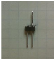
Figure 2.1 Modified 2-pin Header Soldered To Form SDA (DO and DI connection)
