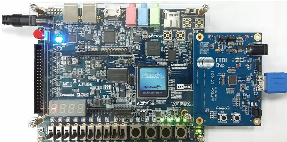
Figure 3.1 UMFT600A/UMFT601A data loopback demo hardware setup
