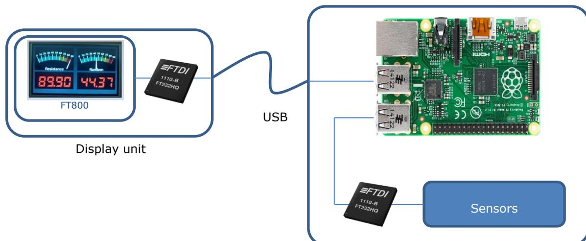
**Figure 2.2 Measurement system**
