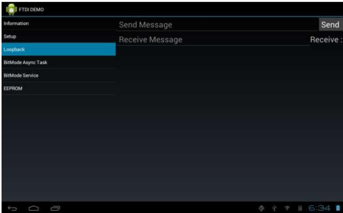
**Figure 4 - D2XX Loopback test running on a tablet**
