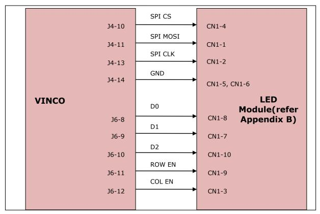
Figure 5 : Interfacing Vinco with LED dot matrix panel
