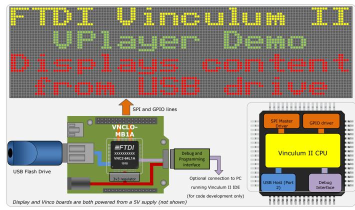
Figure 1 : Vinco Development Module with LED dot matrix display
