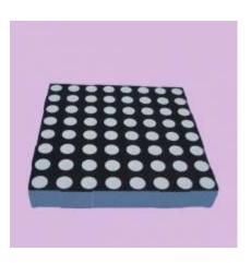
Figure 9 : LED block (8x8 pixels)
