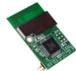
The MC9S08GT60 microcontroller is preprogrammed with DLP Design's Serial Interface Packet Processor (SIPP™ firmware) for accessing the transceiver functions via simple serial calls. Interface to an external serial host microcontroller/ DSP/FPGA, etc. is accomplished via a simple 2-wire (RX, TX, and ground) interface.
