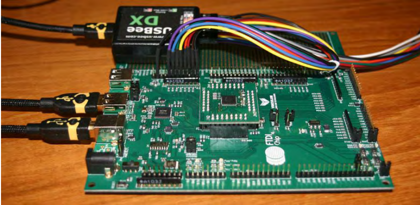
Figure 8.4: Connecting the USBee LA to the V2EvalBoard
