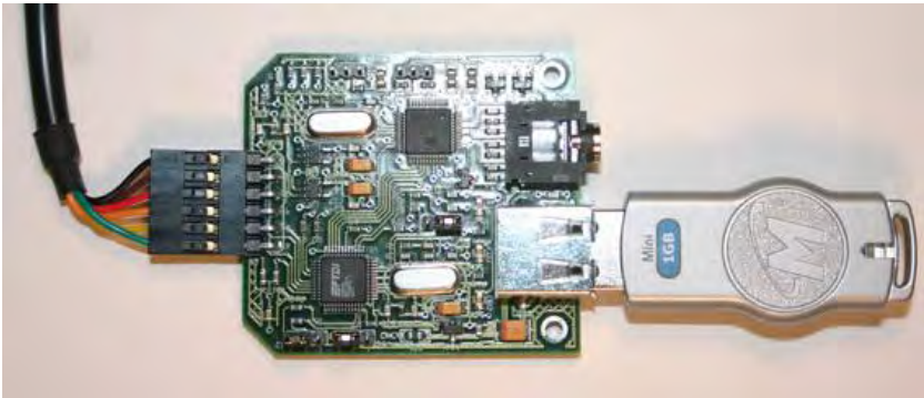
Figure 5.3: USB-to-Serial cable connected to VMusic board
