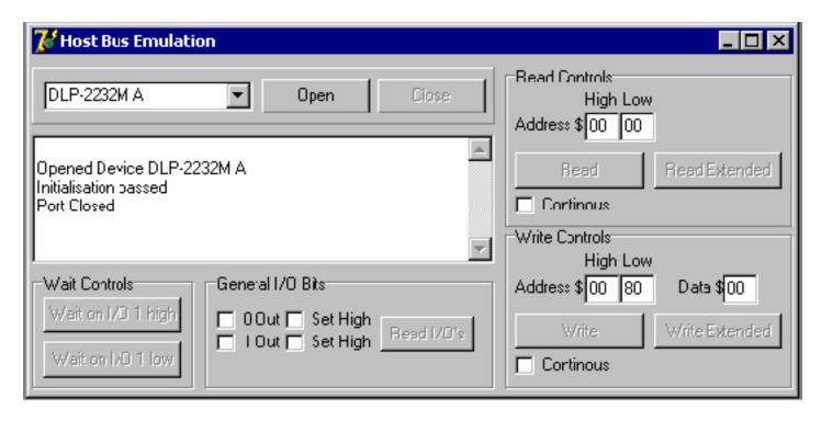
The top left drop down menu allows you to select the device you want to open. In this example device DLP-2232M A was connected.
