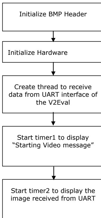
Figure 7: Flow diagram of Windows webcam application
