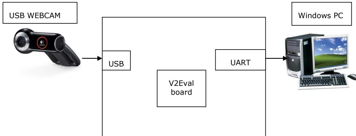
**Figure 1: Connection diagram for webcam demo**
